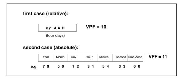
The VP field is given in either integer or semi-octet representation. In the first case, the VP comprises 1 octet, giving the length of the validity period, counted from when the SMS-SUBMIT is received by the SMSC. In the second case, the VP comprises 7 octets, giving the absolute time of the vality period termination.
