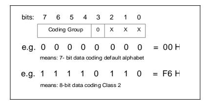
The DCS field indicates the data coding scheme of the UD (User Data) field, and may indicate a message class. the octet is used according to a coding group which is indicated in bits 7..4. The octet is then coded as follows:
